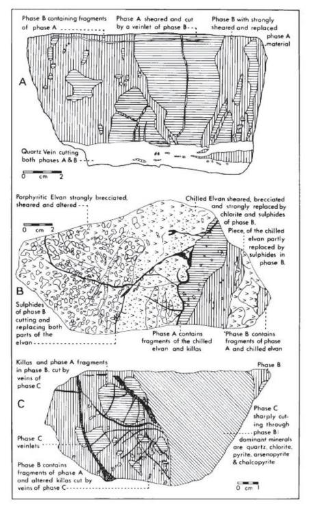
Figure 7.8: Original Drawings of Lode Textures from Mount Wellington Mine
