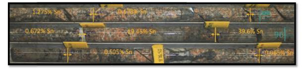
Figure 24.1: No. 4 Lode Mineralised Intercept in SDD20\_001B between 1,034.38m and 1,035.59m down hole
