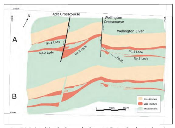
Figure 7.6: Geological Plan View from Level 4 of Mount Wellington Mine, showing observed geology (A) and geological reconstruction (B)
