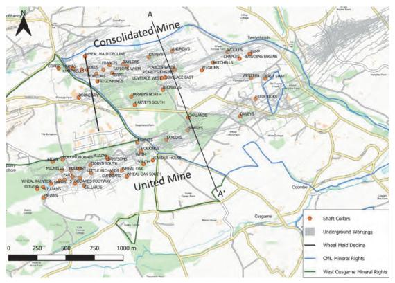
Figure 6.1: Plan View showing the Location of the United and Great Consolidated Mines including the Position of the Main Shafts and section line A-A'
