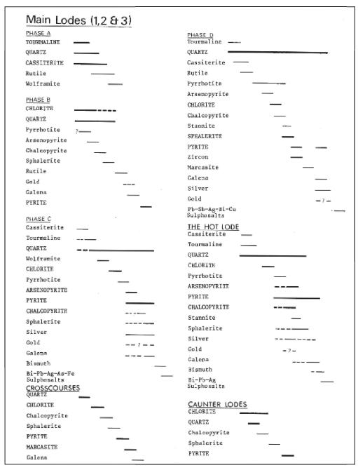
Figure 7.9: Mineralogy and Paragenesis of the Lodes at Mount Wellington Mine After Kettaneh & Badham (1978)
