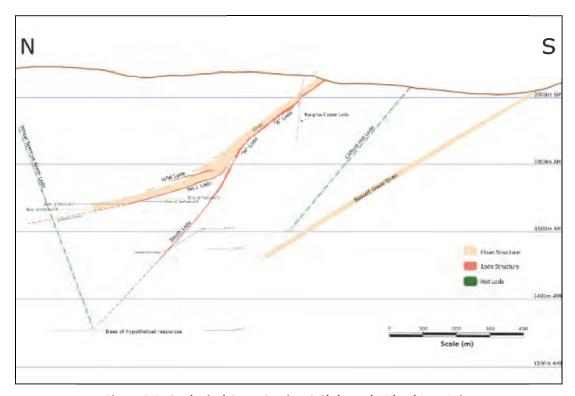
Figure 7.5: Geological Cross-Section C-C' through Wheal Jane Mine
