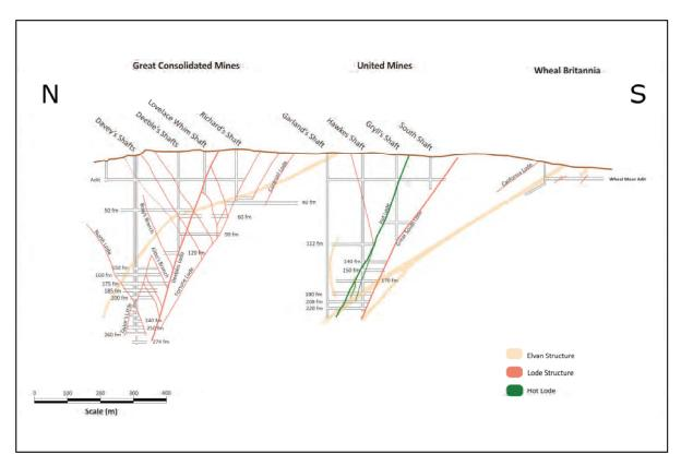
Figure 8: Idealised cross section A-A' through United Mines and Consolidated Mines
