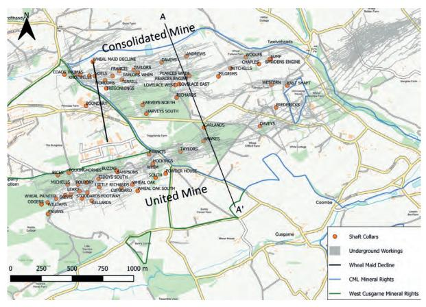
Figure 7: A plan showing the location of the United Mines and Consolidated Mines including the position of the main shafts and section line A-A'
