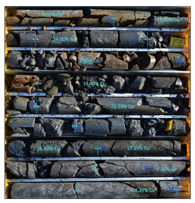
Figure 10: Mineralised intersection in GWDD-002 from 93.48m to 101.05m downhole
