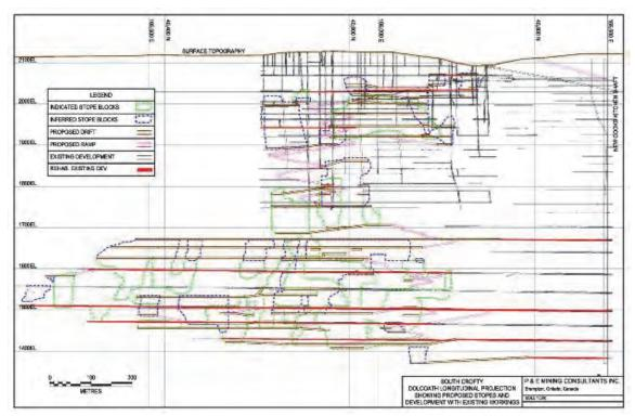
Figure 24.3: Longitudinal Projection of the South Crofty Dolcoath Section Underground Mine
