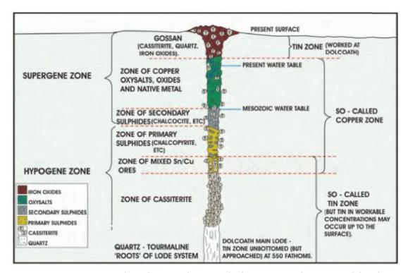
Figure 8.2: Cross-Section Through a Typical Sn-Cu Lode showing Vertical Zonation Exhibited in some Major Structures (Hosking 1988).
