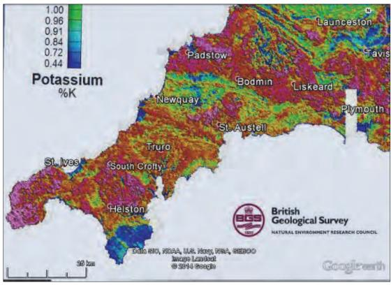
Figure 7.2: Airborne Radiometric Map of southwest England showing Potassium (K) Distribution (British Geological Survey "TELUS SW Project" overlain on Google Earth 2014.)
