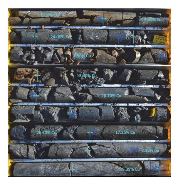
Figure 10.2: Mineralised Intersection in GWDD-002 from 93.48m to 101.05m Down Hole
