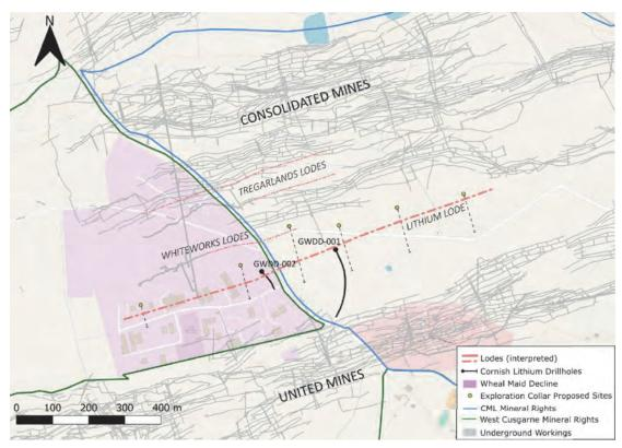
Figure 10.1: Collar Locations of Drill Holes GWDD-001 and GWDD-002
