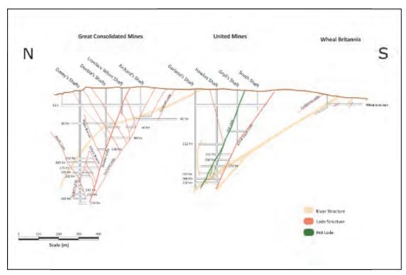
Figure 6.2: Idealised Cross-Section A-A' through United and Great Consolidated Mines
