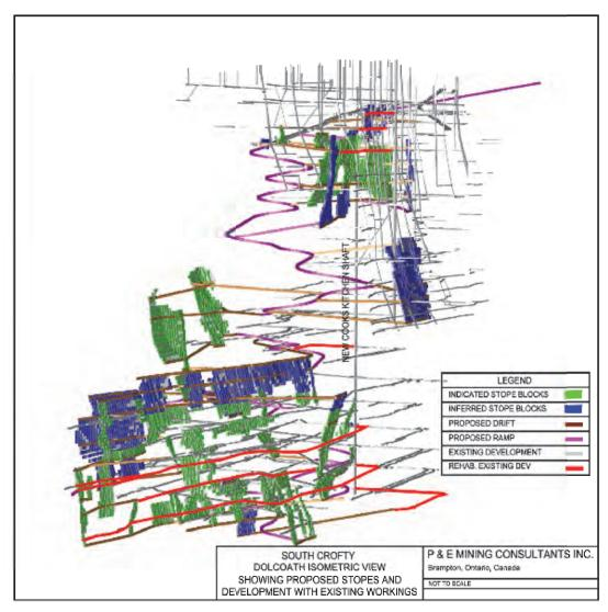
Figure 24.2: Isometric View of the South Crofty-Dolcoath Section Underground Mine Layout
