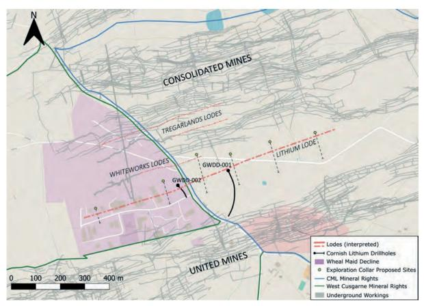
Figure 9: The collar locations of drill holes GWDD-001 and GWDD-002
