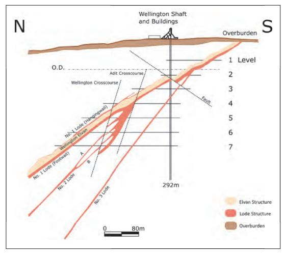
Figure 7.4: Cross-Section line B-B' from the Mount Wellington Mine
