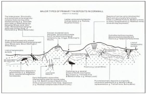
Figure 8.1: Primary Tin Deposits in Cornwall (after Hosking 1988)
